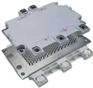
H4 Package Pinfin(140 x 72 x 25.4mm)
